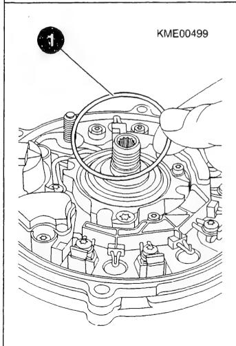
DISMANTLING AND CHECKING ALTERNATOR Dismantling adhesive ring at regulator NOTE: This work need not be performed if regulator is replaced. Carefully prise adhesive ring (1) off regulator (2) at straight edge (see Fig.).
